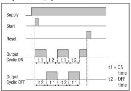
Typical application of Continuous start and reset in On delay mode:
