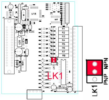
The Digital inputs can be configured as PNP inputs. This means that the inputs can be operated by switching to +12V to +24V. Open the IO Module. Change the link **LK1** to the PNP position as shown below.
